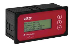
The display shows the lowest scanned input that de-energized the safety outputs (safety outputs open). After the lowest scanned input is cleared, the display will refresh and show the next input which is open. In this way, each open input circuit can be troubleshot and closed. When all inputs are closed, the user can scroll through the display.
